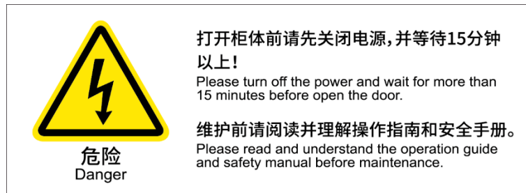
Figure 2-6 Open door power off &amp; maintenance sign
