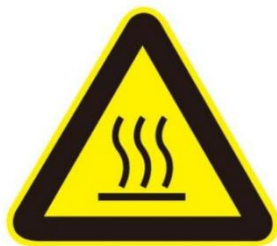
Figure 2-8 High temperature mark
