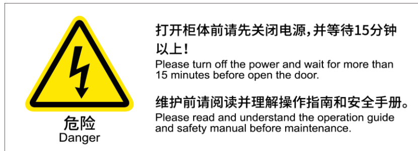
Figure 1-7 Door-opening power-off & maintenance signboard
