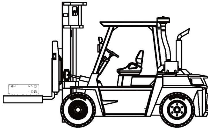
Figure 2-1 Schematic diagram of control cabinet transportation by forklift
