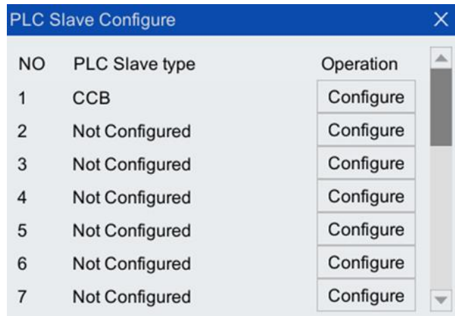
Fig. 2-16 "PLC Slave Configuration" floating window
