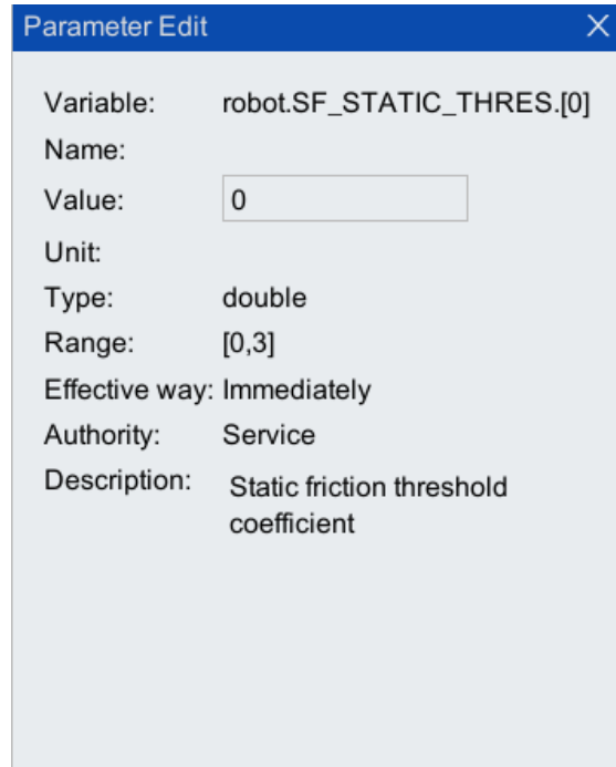
Figure 4-11 Configuration interface of static friction threshold coefficient
