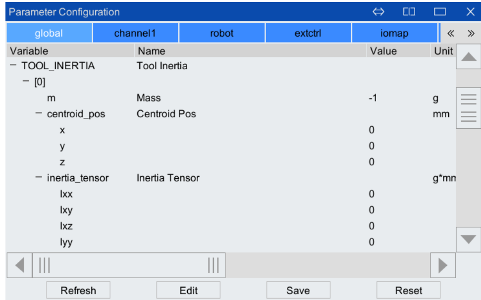
Figure 4-5 Tool inertia parameter setting interface
