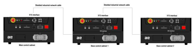
Figure 2-7 Connection diagram of three inCube10/12 control cabinets
