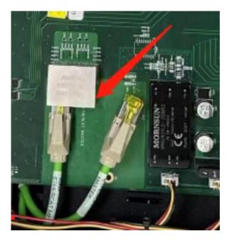
Figure 2-15 Ethercat Network Cable Location Map on DCBS Board
