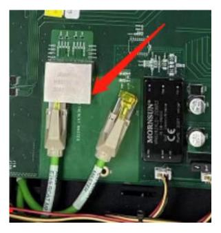
Figure 2-11 EtherCat Network Cable Location Map on DCBS Board
