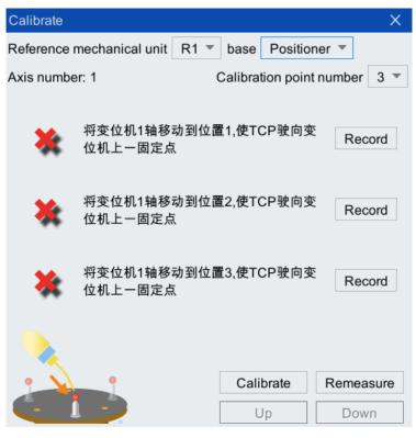
Figure 4-41 Calibration interface
