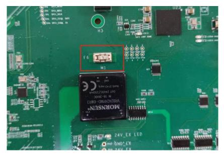
Figure 2-14 Location diagram of F6 fuse on MCBS board
