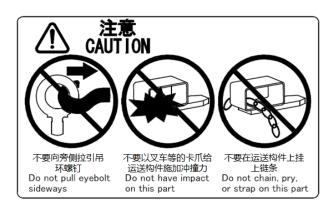
Figure 9-1 Precautions for manipulator during handing
