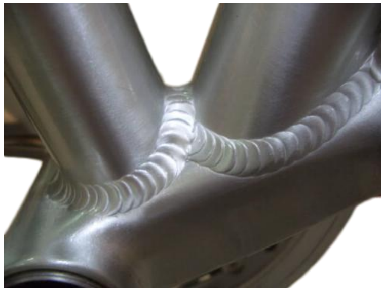
Figure 7-36 Fish scale welding effect diagram
