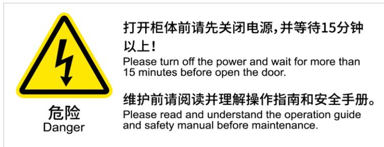
Figure 1-6 Door opening and power-off & maintenance indicator
