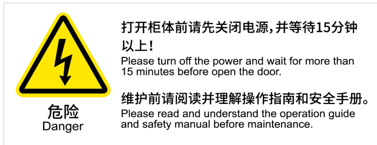
Figure 1-6 Door opening and power-off &amp; maintenance indicator
