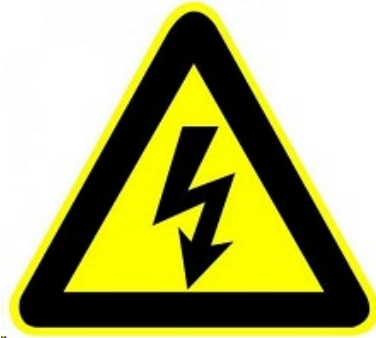
Figure 1-8 Electric shock sign
