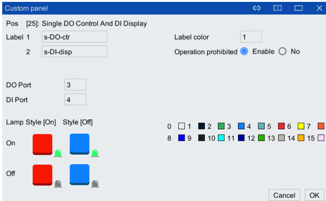
Figure 6-101 "Single DO control and DI display" Setting interface
